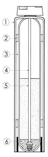
Figure 14: Resin Tank Assembly
