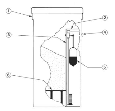
Figure 10: Standard Brine Tank Assembly (25, 25CX, 35, and 48)
