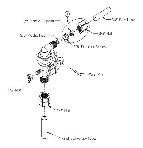
Figure 23: Brine Valve Elbow Installation
