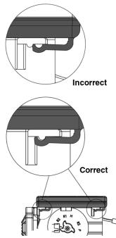
Figure 9: Controller Tab Lock Detail
