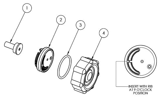
Figure 19: Injector Assembly
