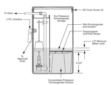
Figure 13: Potassium Permanganate Feeder (P/N PT1424)
