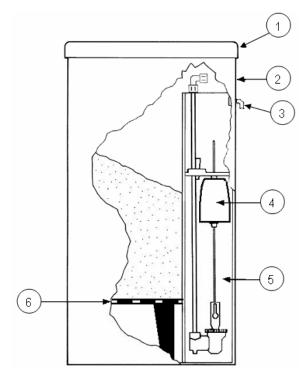
Figure 12: Optional Brine Tank Assembly
